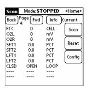
Page 4 contains some fuel-specific parameters. FTC is the fuel trim cell number, followed by O2 voltages, short & long-term fuel trims, and closed-loop status.
